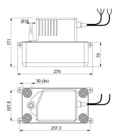
The accessory is supplied in kit form and involves the installation outside the machine of a condensate booster pump equipped with a tank with a microswitch float switch to activate the pump.
