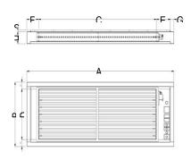
Motorised ON/OFF non-return air damper positioned above the unit in both UNDER and OVER versions.
