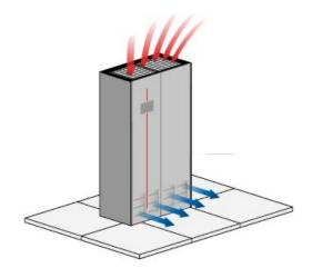
Available for UNDER versions, the accessory provides a grille to front panel to ensure front air delivery, we recommend the combination with a plenum with grille to improve system performance.
